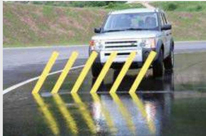
Miniature shock absorbers protect the end positions during driving safety training
