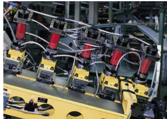
Stamping units placed in line
