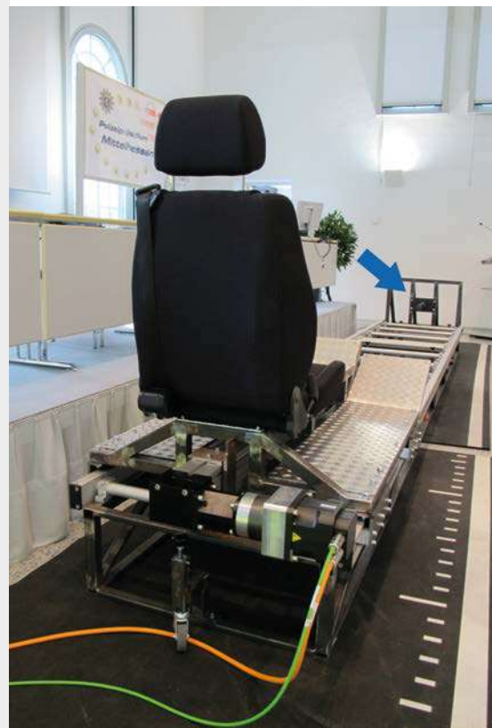
MAGNUM dampers ensure the reliable braking of moving masses on the seat and the protection of the entire carriage construction Central Hessian Police Department, Karl-Glöckner-Straße 2, 35394 Gießen, Germany
