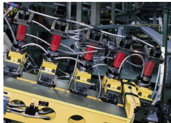
Stamping units placed in line
