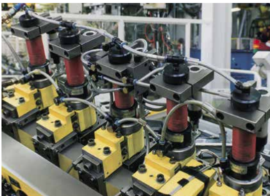
Stamping units placed in line
