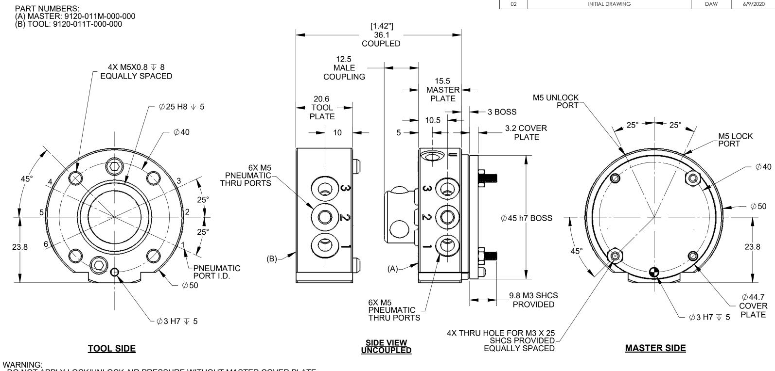
DO NOT APPLY LOCK/UNLOCK AIR PRESSURE WITHOUT MASTER COVER PLATE PROPERLY ATTACHED. IF COVER PLATE IS NOT USED, MASTER SHOULD BE PROPERLY ATTACHED TO INTERFACE. FAILURE TO DO SO COULD RESULT IN DAMAGE TO COVER PLATE AND O-RING.
