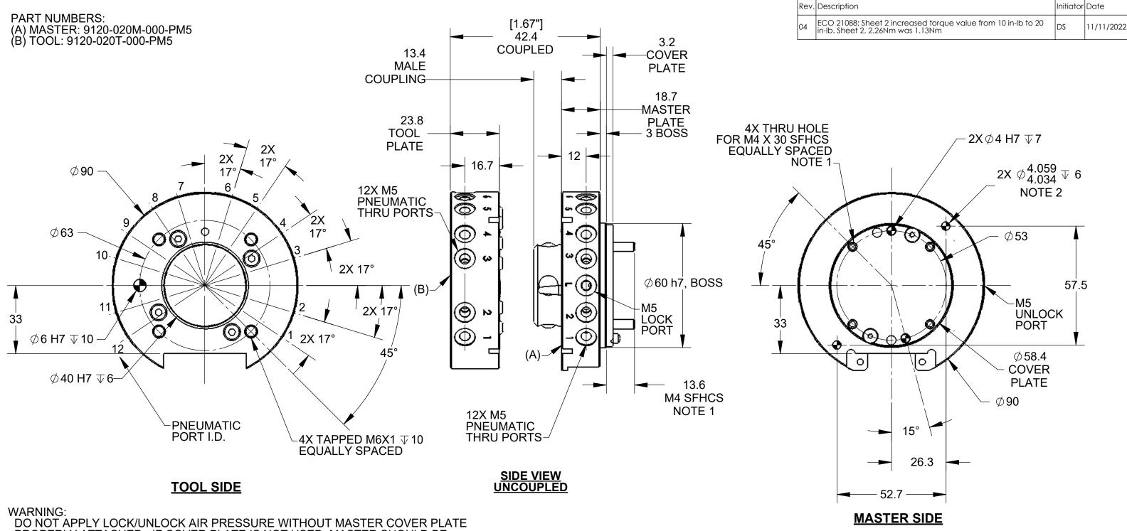
PROPERLY ATTACHED. IF COVER PLATE IS NOT USED, MASTER SHOULD BE PROPERLY ATTACHED TO INTERFACE. FAILURE TO DO SO COULD RESULT IN DAMAGE TO COVER PLATE AND O-RING.
