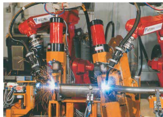
Welding fixture for exhaust components
