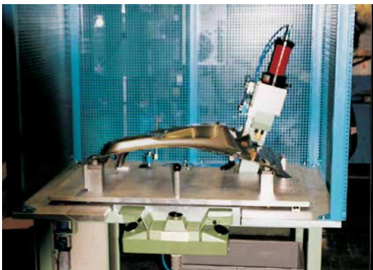
Device for holes Ø 8 in sheet metal
