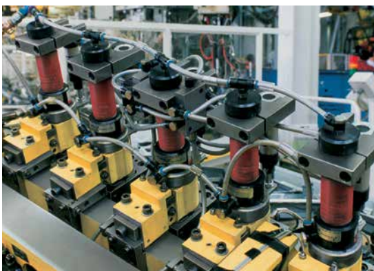
Stamping units placed in line
