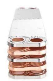
A brazed plate heat exchanger (BHE) is very compact compared to other heat exchangers for similar applications, meaning less refrigerant is needed. AlfaNova is a range of fusion-bonded, all-stainless-steel heat exchangers. They are ideal in situations involving media that is corrosive or very sensitive to contamination of copper or nickel.
