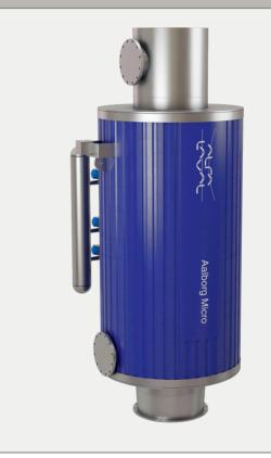
The Alfa Laval Aalborg Micro is a uniquely compact boiler/ economizer designed for waste heat recovery from a vessel's auxiliary engines. Easy to install, operate and maintain, it reduces the use of the oil-fired boiler by reclaiming heat that otherwise would be lost through the exhaust gas.
