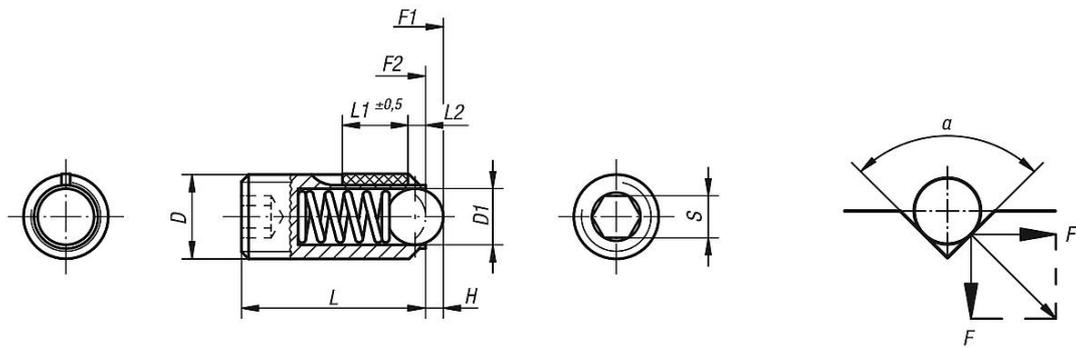
$$\begin{aligned} \alpha = 60^\circ, F' &= 1,732 \times F \\ \alpha = 90^\circ, F' &= F \\ \alpha = 120^\circ, F' &= 0,577 \times F \end{aligned}$$
