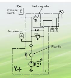
The pressure switch, accumulator, filter kit, and reducing valve are options. Select these options according to your application.
