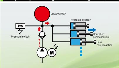
When the pressure switch reaches its upper limit, it stops the motor. The hydraulic pressure that is accumulated in the accumulator maintains the pressure in the circuit (compensates for cylinder operation and compensates for leak while maintaining pressure), and when the pressure switch reaches its lower limit, it starts the motor again. (Use the pressure switch signal to start and stop the motor.)
