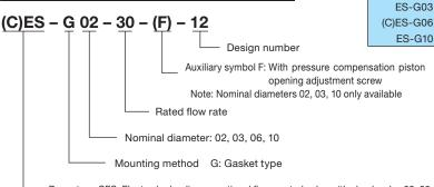
Pump type CES: Electro-hydraulic proportional flow control valve with check valve 02, 06 only ES: Electro-hydraulic proportional flow control valve
