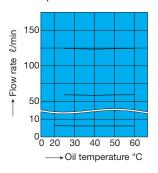
Supply Pressure Load Pressure 14MPa 10MPa Operating Fluid VG32 Value when a Nachi-Fujikoshi special amplifier is used (with dithering).
