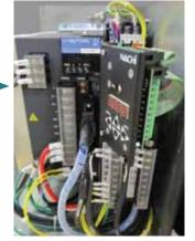
The rotary switch has 1~9 and A~F channels. It is also available to select 16 patterns by setting parameter. (Manual operation mode)
