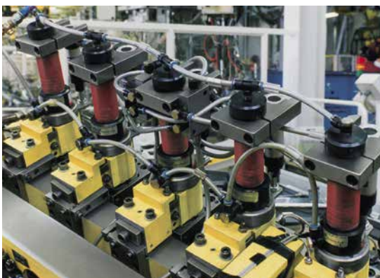
Stamping units placed in line
