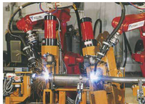
Welding fixture for exhaust components
