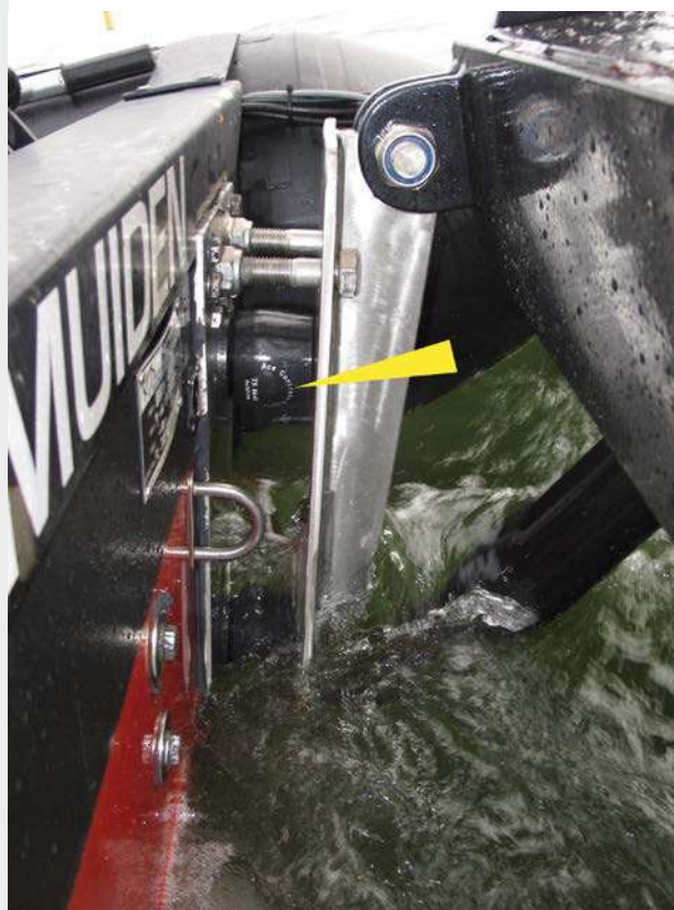
Seawater-resistant, robust TUBUS profile dampers made of co-polyester elastomer allow boats and crew to dock safely Wals Diving and Marine Service, 1970AC IJmuiden, Netherlands
